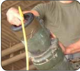
Tube Strip being inserted into a barrel.
