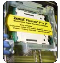
1" x 3" Plastab in an electronic's enclosure
